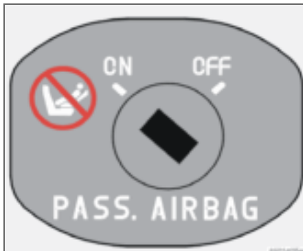
Switch for SRS in ON position.
