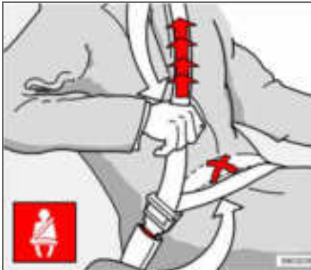
Tensioning the hip strap. The belt must be positioned low down.
